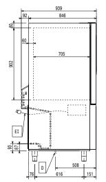
Drain Electrical inlet (power)
